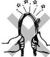
Do not bend insertion tube in a tight radius, as this will damage delicate fiber bundles.
