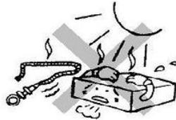
Direct sunlight, dust, high humidity and high temperature will damage instruments.
