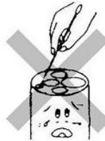
Do not use a needle or other sharp object to remove debris from air/water nozzle. The nozzle may be deformed or pried loose.
